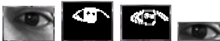
Fig. 1. Steps for extracting smaller eye regions. Left to right: Input image, p -tile thresholding, dilation result, and the final cropped eye region.
