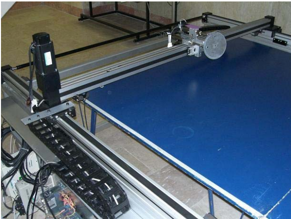
Figure 9. The ping-pong player robot, Robo-Pong.
