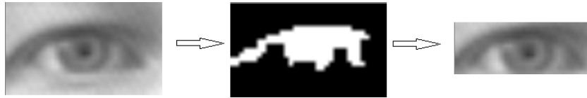
Fig. 2. Example for finding a smaller eye region.
