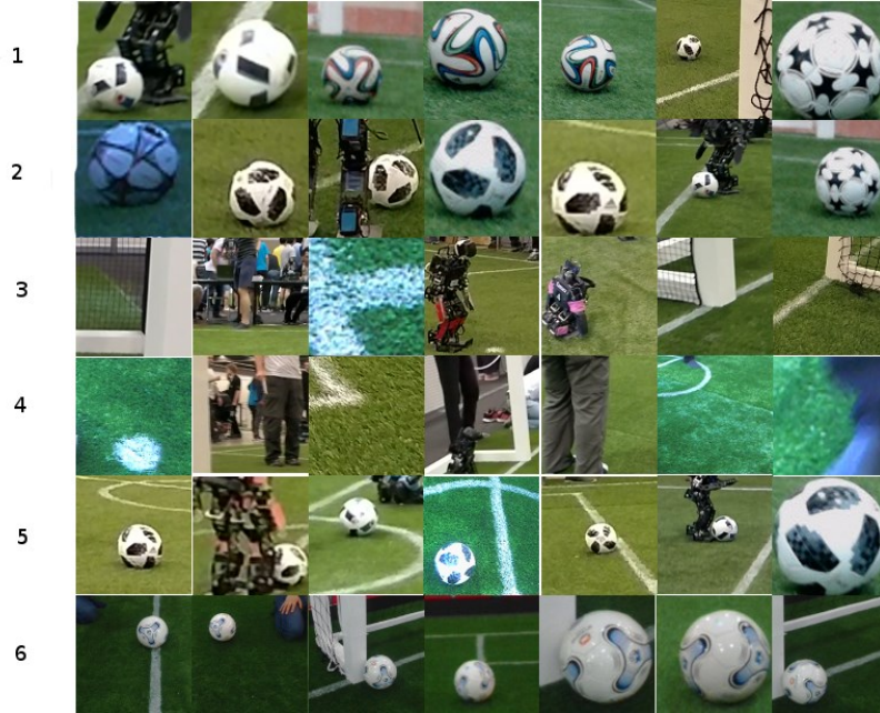
Fig. 3. Row 1, 2: Positive samples in the training data set. Row 3 and 4: Negative samples in the training data set, Row 5: Positive samples of the validation data set. Row 6: Positive samples of generalization data set with a new ball pattern not used for training.
